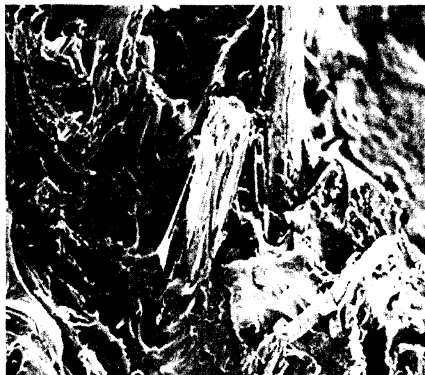
Fig. 5. SEM micrograph of the tensile fracture surface of PP-kenaf (20%) without MAPP.
