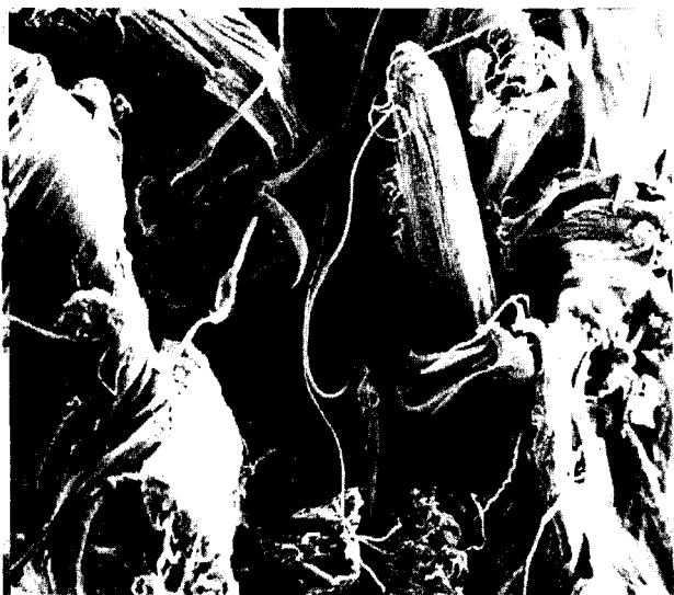
Fig. 4. SEM micrograph of the tensile fracture surface of PP-kenaf (20%) with MAPP.
